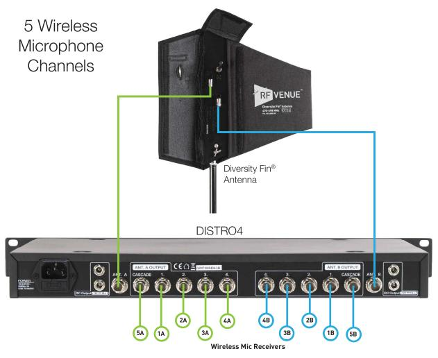
\*Please note - 4 DC ports are provided for powering receivers, for a fifth receiver, external power supply required.
